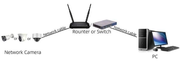
Figure 1-2Connecting via a Switch or a Router
