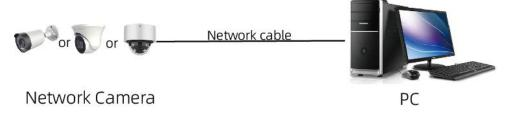
Figure 1-1 Connecting Directly
